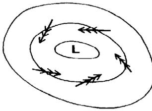
The surface wind around a low pressure points to the low pressure by about 30° over land due to the friction. This effect is less over the sea where the friction is less.
