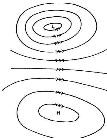
The coriolis force means that in the Northern Hemisphere, the geostrophic wind circulates anticlockwise round a low and clockwise round a anticyclone (high pressure). The winds rotate in the same direction as the isobars, but this is only true for winds at altitude (over about 1,000ft). The effect of the ground causes friction which slows down the surface winds.
